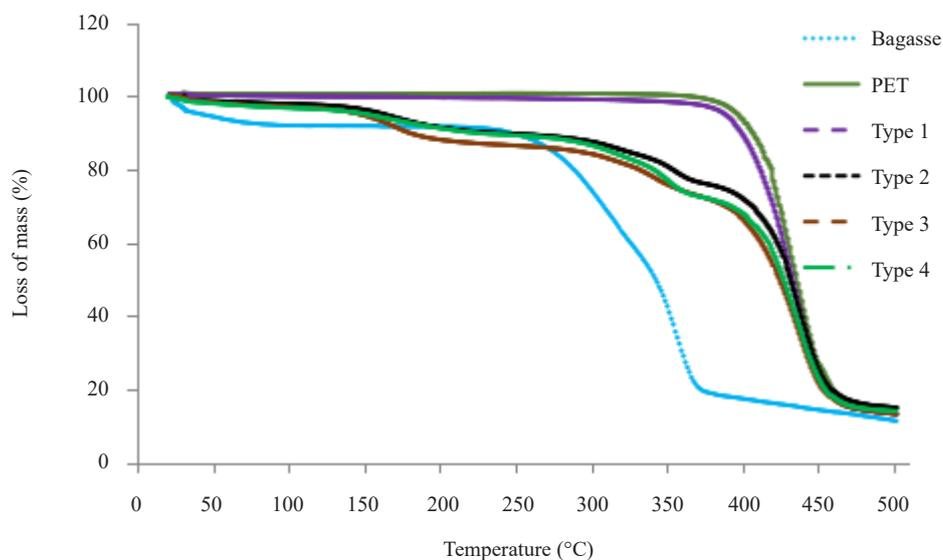
**Figure 2.** Thermogravimetric analyses of all samples
