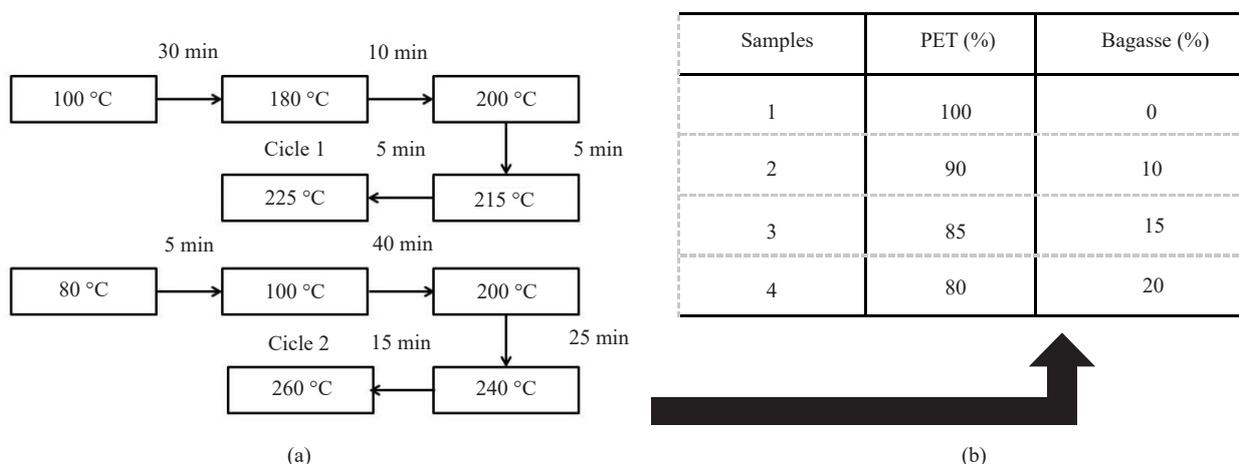
Figure 1. (a) Temperature cycles 1 (PET) and 2 (PET/Bagasse Fiber), (b) Composition of samples
