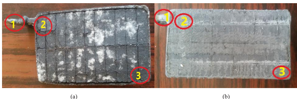
Figure 2. (a) Removed Anode plate after explosion of battery, (b) Removed cathode plate after explosive of the battery
