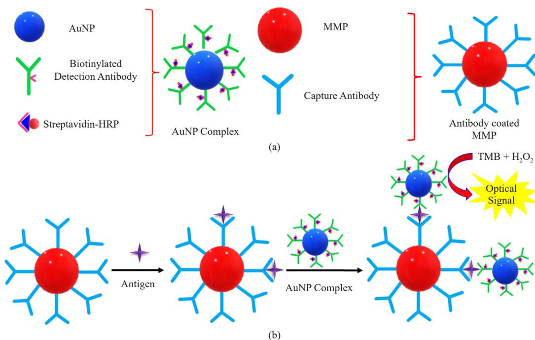
**Figure 16.** Development of antibody-coated MMP based (a) AuNP-anti-CEA-HRP complex, and (b) AuNP complex based on colorimetric enzyme immunoassay route<sup>66</sup>
