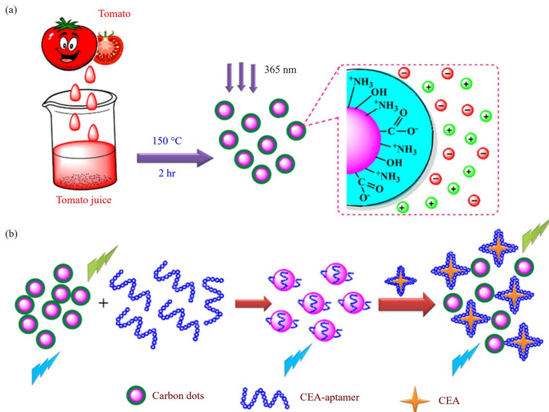
Figure 19. synthetic routes of (a) carbon dots (CDs), and (b) assay CEA via CDs<sup>71</sup>
