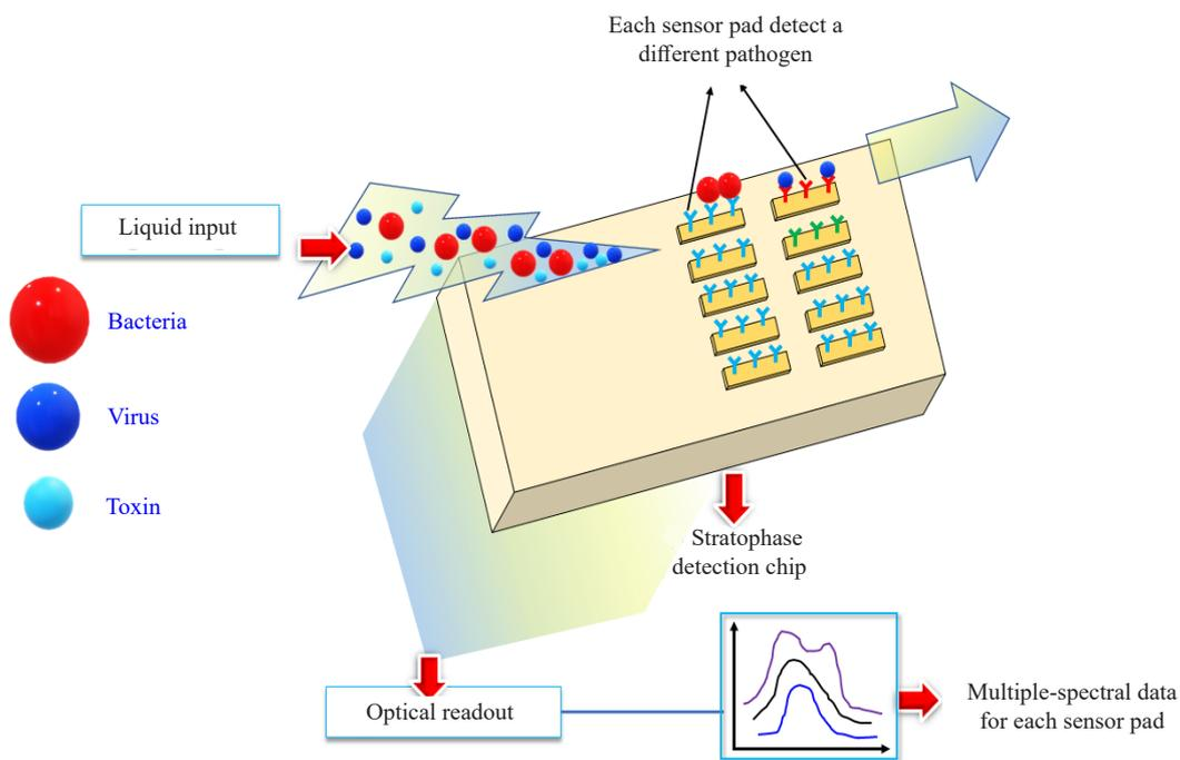
Figure 9. Schematic representation of optical biosensor<sup>57</sup>
