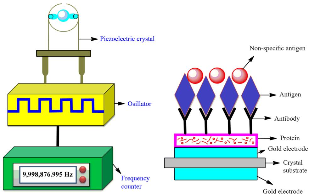
Figure 10. Piezoelectric biosensor demonstrated antibody-antigen binding<sup>58</sup>
