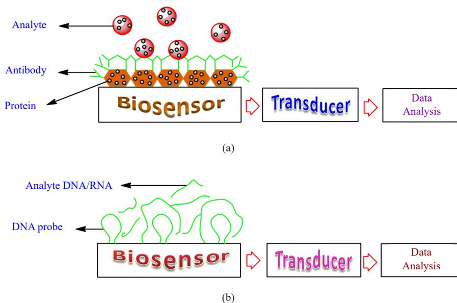
Figure 5. Schematic representation of biosensor detection process<sup>43</sup>
