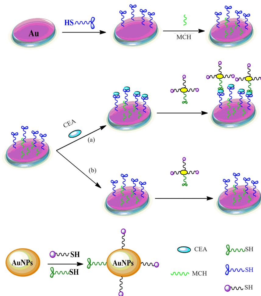
**Figure 15.** Schematic representation of AuNPs signals amplification electrochemical aptamer biosensor identification of CEA<sup>65</sup>
