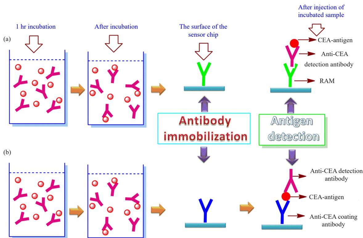
Figure 17. Schematic demonstration of (a) homogenous RAM-capture, and (b) sandwich assay<sup>69</sup>
