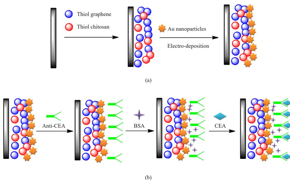
**Figure 13.** Schematic representation preparation of immunosensor: (a) nanocomposites film, and (b) CEA immunosensor<sup>63</sup>
