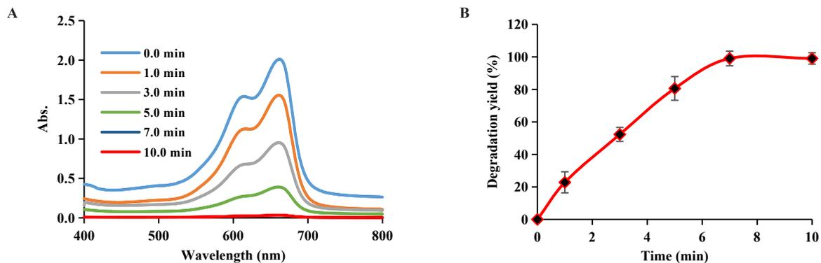
**Figure 3.** (A) UV-Visible spectra of 20.0 mg L<sup>-1</sup> MB at different times (in the unit of min) and (B) the effect of time on the nanozyme-mediated methylene blue degradation. Error bars are represented in 3 replicate experiments
