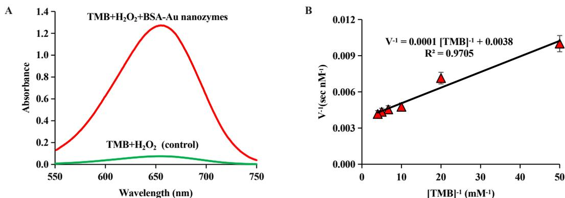
**Figure 2.** (A) The peroxidase-like activity of the as-prepared nanozymes vs. control sample (TMB + H<sub>2</sub>O<sub>2</sub>) and (B) Lineweaver-Burk plot for calculating the kinetics parameters of the as-prepared nanozymes
