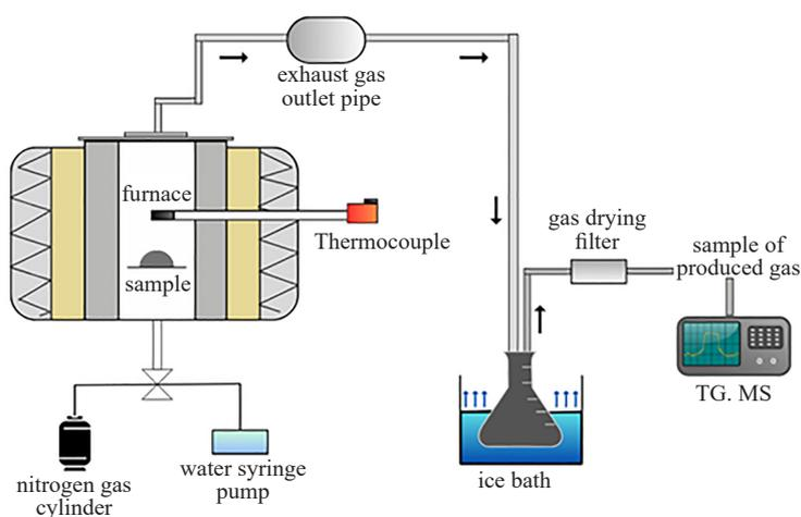
Figure 1. Schematic diagram of experimental set up
