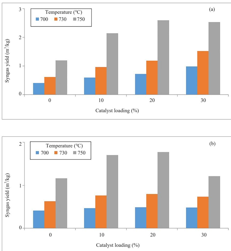
**Figure 4.** Effect of catalyst loading and temperature on syngas yield at Ca/C = 1 for (a) K<sub>2</sub>CO<sub>3</sub> and AP char and (b) CeO<sub>2</sub> and AS char
