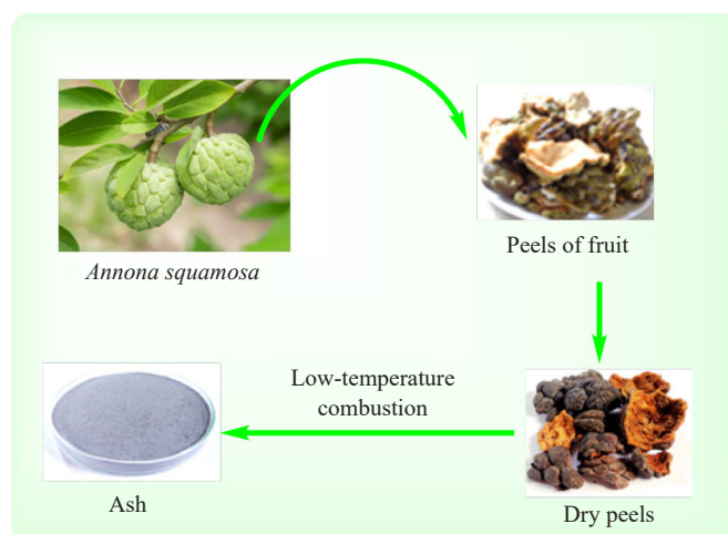
Figure 3. Preparation of the sugar apple peels ash catalyst
