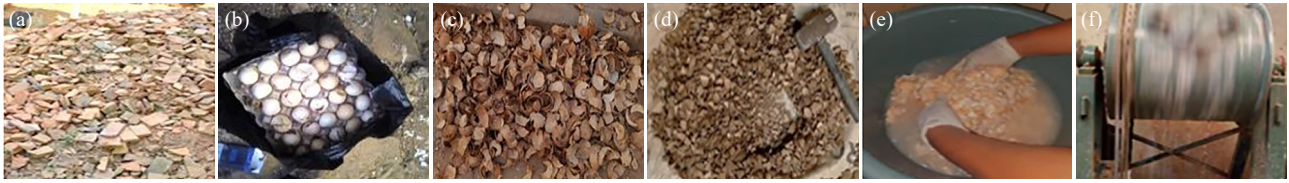
Figure 1. Raw materials (a) Collection of grog (b) eggshell (c) coconut shell (d) crushed coconut shell (e) washing of eggshell (f) grinding of raw materials
