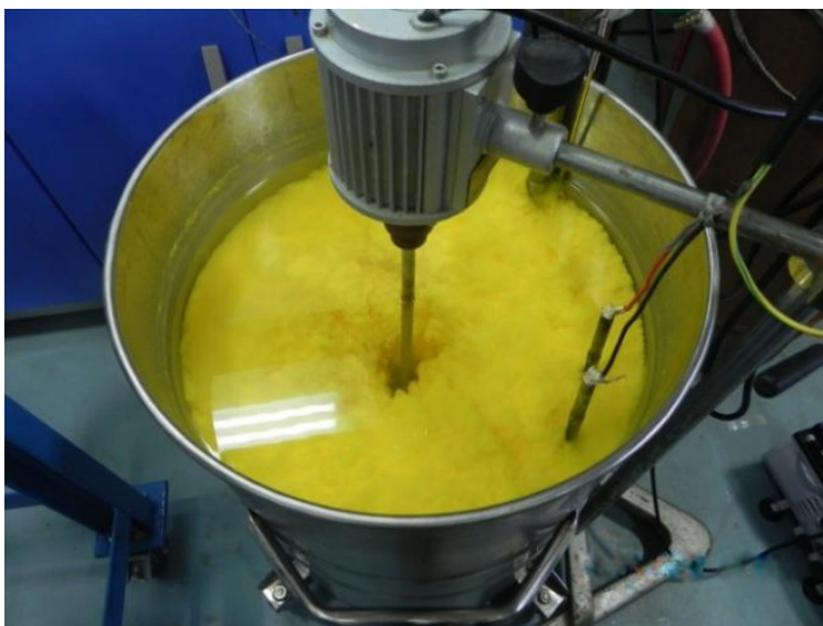
Figure 13. Precipitation of U from stripped solution after purification through HNO 3 -TBP route as ADUC using air-ammonia mixture
