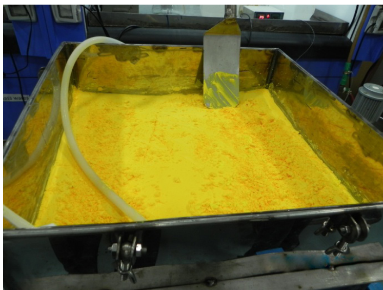
Figure 14. Filtration of nuclear grade ADUC using pan filter under vacuum
