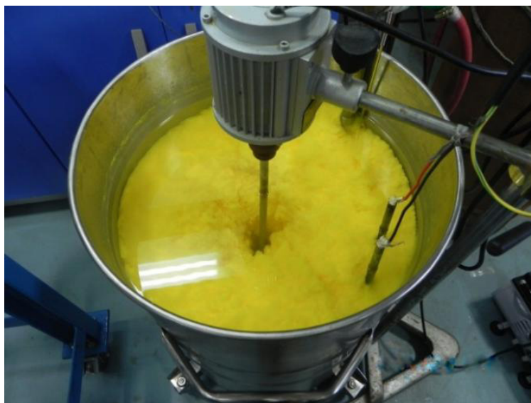
Figure 13. Precipitation of U from stripped solution after purification through \text{HNO}_3 -TBP route as ADUC using air-ammonia mixture
