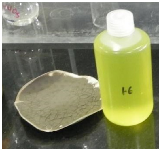
(b) Residue and uranyl sulphamate solution
