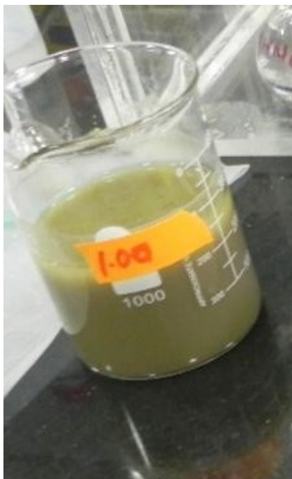
(a) SDU in sulphamic acid solution
