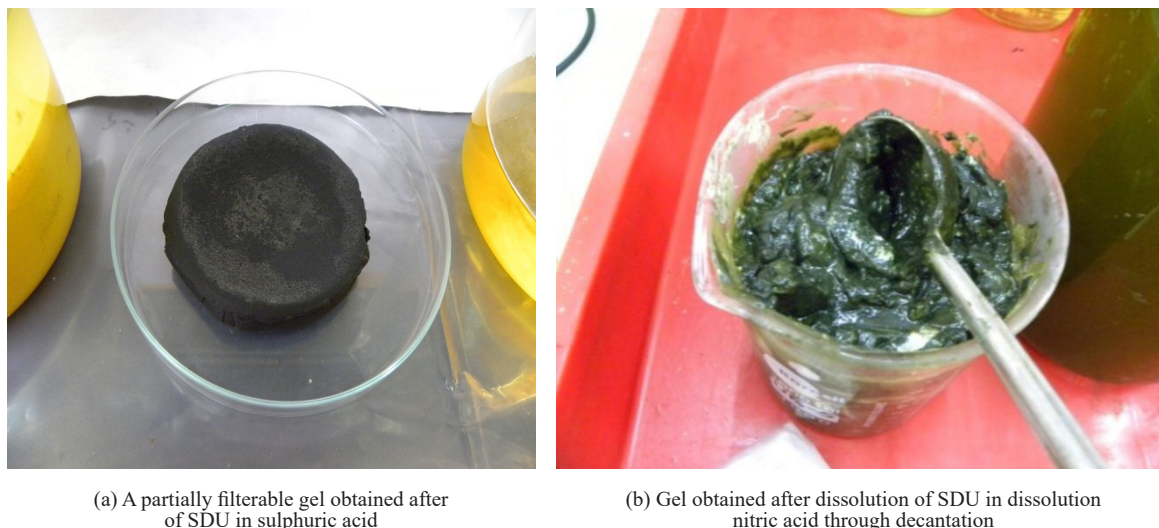
Figure 7. Gel formation during dissolution of crude SDU in different acids
