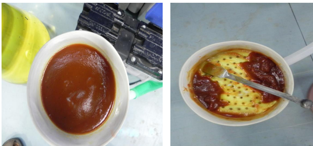
Figure 10. Acid insoluble obtained after dissolution of U 3 O 8 (obtained by calcination of Ammonium Di-Uranate) in nitric acid medium
