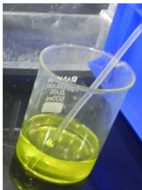
(d) Uranyl nitrate solution after dissolution of Ammonium Di-Uranate in \text{HNO}_3
