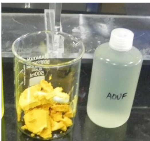
(c) Ammonium Di-Uranate and filtrate
