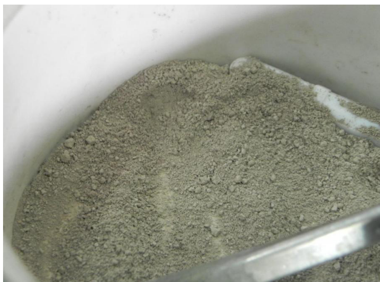
Figure 9. Silica/silicate, Zr and Polyacrylamides separated from crude SDU dissolved in sulphamic acid
