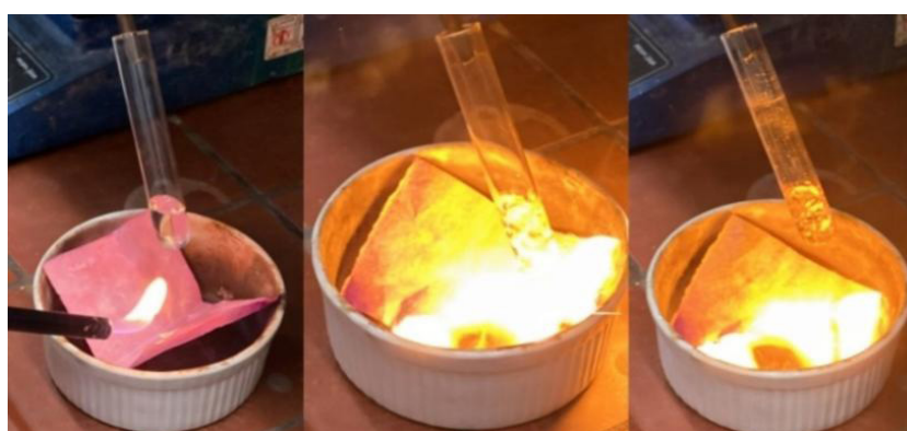
Figure 9. Low-boiling acetone brought to reflux (middle & right photos) by heat released from the combustion of cobalt acetate-impregnated flash paper, serving as a small-scale analogue for steam generation in turbine-driven electrical systems. The photo on the left shows acetone solvent at room temperature prior to igniting the impregnated flash paper
