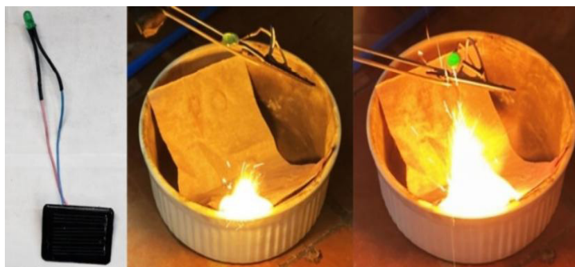
Figure 10. Alternative harvesting of thermal energy from the self-sustained combustion of cobalt acetate-impregnated flash paper. From left to right: a mini silicon photovoltaic directly converts the intense heat and light into electricity, illuminating the green LED as it approaches the burning surface
