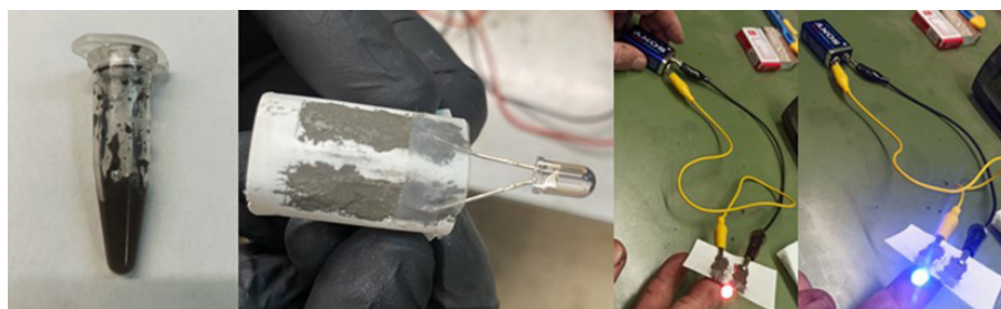
Figure 4. From left to right: conductive silver paste prepared from derived silver metal and water glass (70% Ag); application of the paste onto paper using a small brush to form two parallel conductive traces, along with attachment of an LED at one end of the traces using tape; connection of a 9 V battery at the opposite end via clips, resulting in illumination of red or blue LEDs
