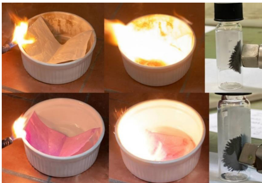
Figure 5. Rapid flash-paper combustion synthesis of nickel (top row) and cobalt (bottom row). From left to right, each sequence depicts the ignition of flash paper impregnated with either nickel acetate or cobalt acetate, leading to a bright, self-sustained combustion reaction. The images on the right display the resulting magnetic metals collected inside vials, visibly attracted to the side by a strong external magnet
