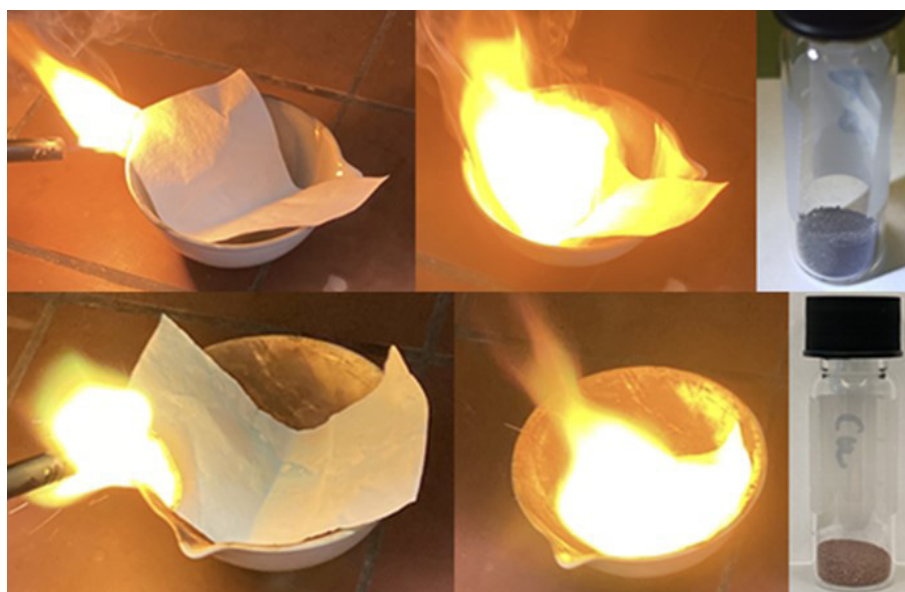
Figure 1. Flash-paper combustion synthesis of silver (top row) and copper (bottom row). From left to right, each sequence shows ignition of flash paper impregnated with silver nitrate or copper nitrate, respectively. Ignition initiates a self-sustaining exothermic reaction, driving rapid decomposition of the metal nitrate and resulting in the formation of elemental silver or copper. The vials on the right show the collected metallic products after completion of the reaction
