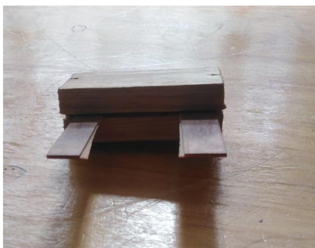
Figure 2. Copper plates overlaid on the GO/NCC composite material
