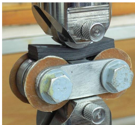
Figure 1. Process of specimen failure by interlaminar shear in test machine
