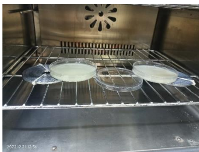
Figure 7. CNC suspension in petri dish, in an oven. It illustrates the process of forming a CNC film. Initially, the CNC suspension is placed on a petri dish inside an oven. As the temperature is raised, the CNC suspension evaporates, resulting in the formation of a film. A PFO is positioned below the petri dish during this process
