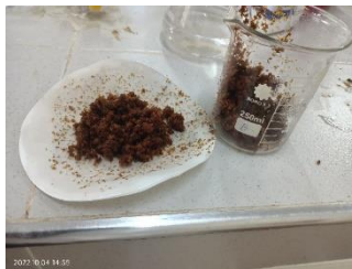
Figure 1. Coffee husks after alkaline treatment with NaOH. The image depicts coffee husks following treatment with NaOH, resulting in a notable transformation in color to dark brown. This change is attributed to the process of de-lignification and the removal of hemicellulose, which are key steps in the alkaline treatment procedure. The dark brown hue observed in the treated coffee husks signifies the successful alteration of their chemical composition, indicative of potential modifications in their structural properties.
