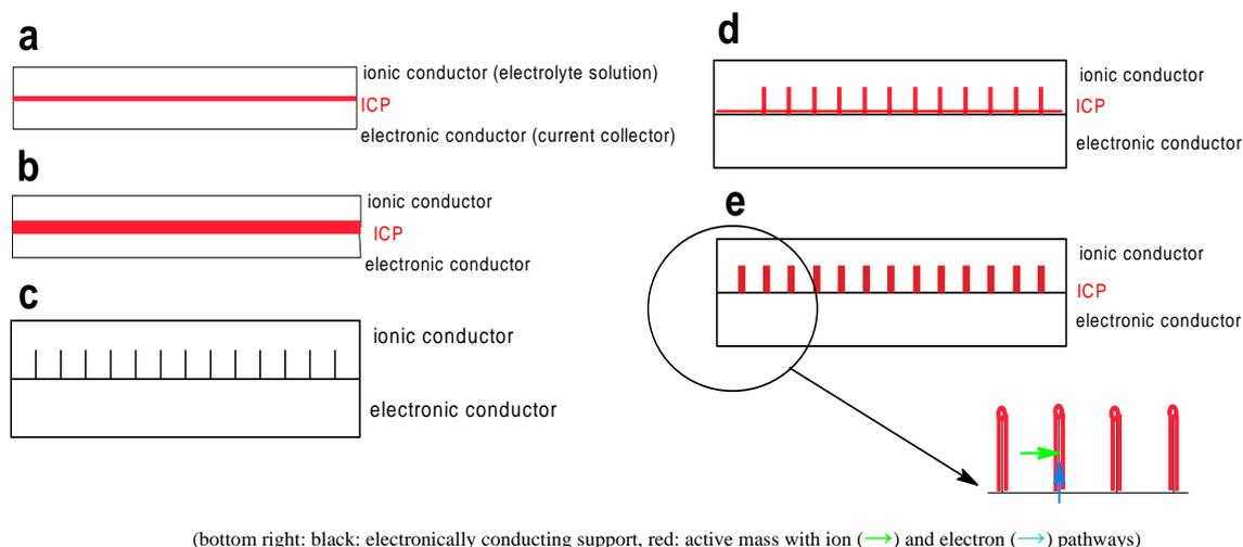
**Figure 2.** Schematic supercapacitor electrode architectures, for details of subfigures see text.
