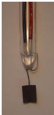
Figure 3. A dynamic hydrogen reference electrode according to Giner
