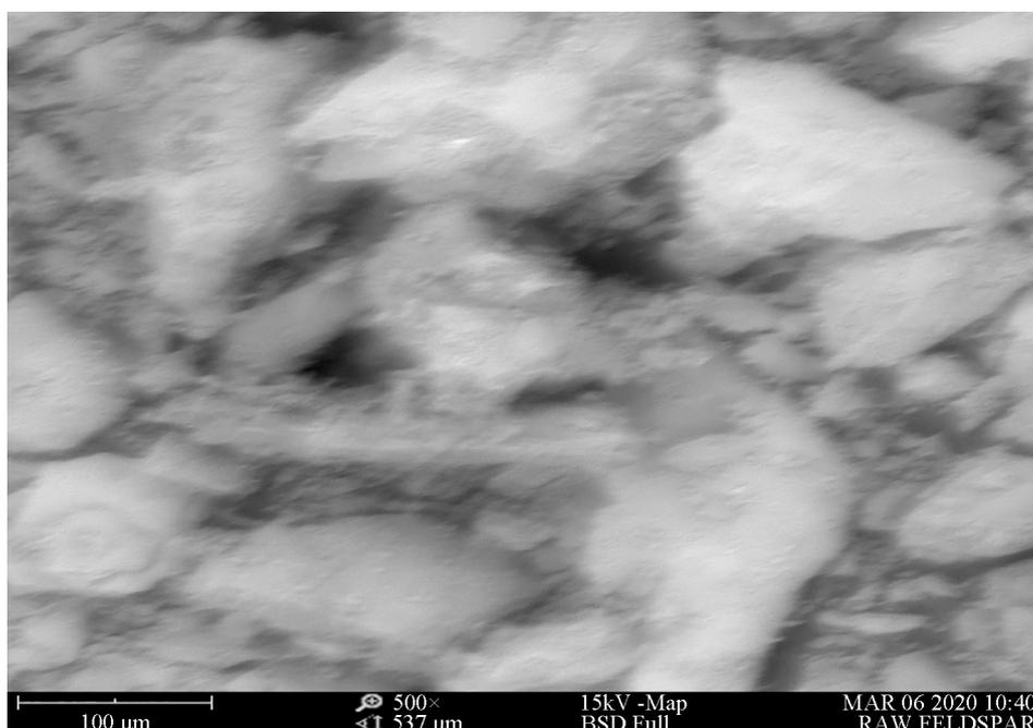
Figure 6. SEM of raw feldspar adsorbent at a magnification of (500X)
