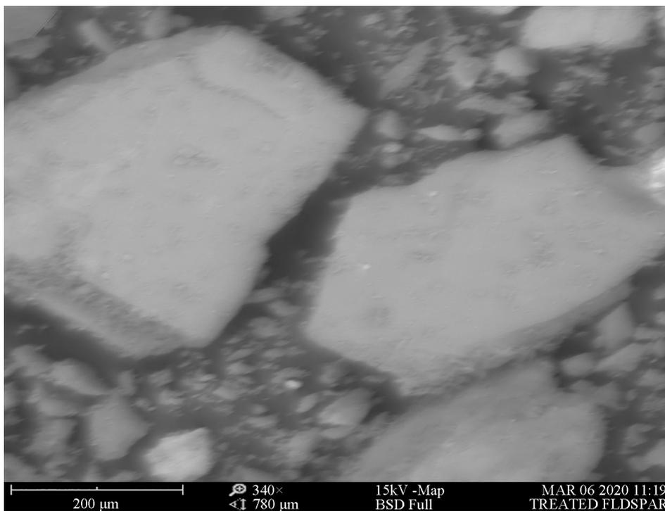
**Figure 7.** SEM of treated feldspar adsorbent at a magnification of (340X)
