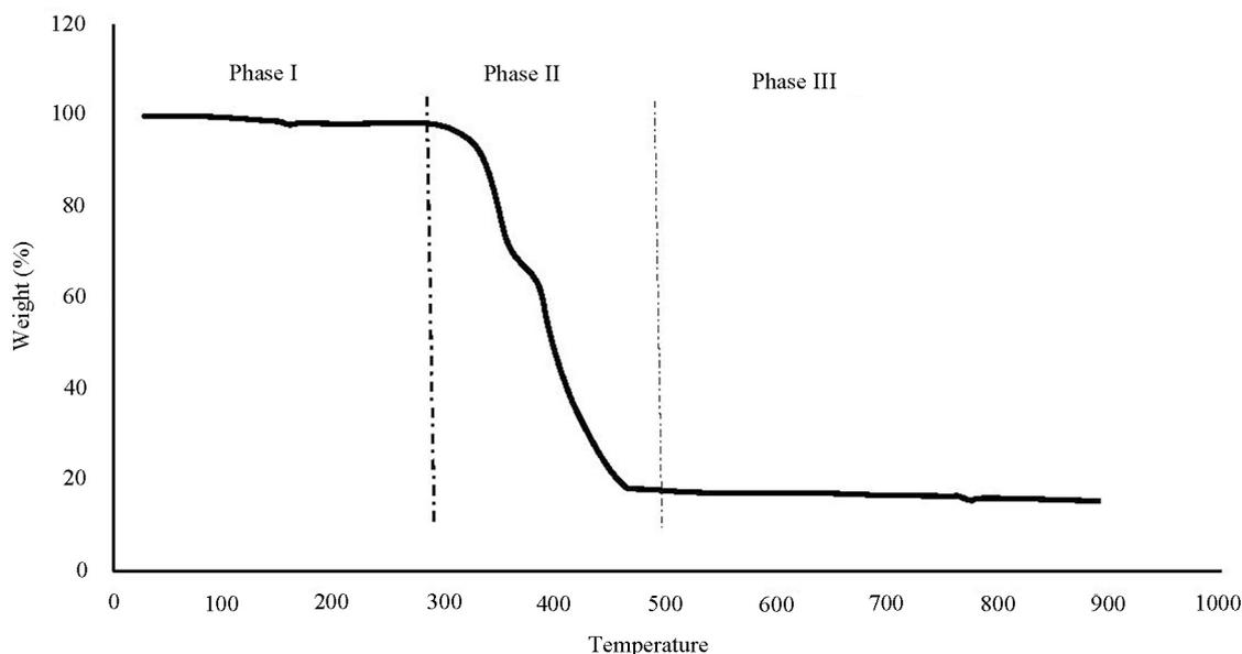
**Figure 3.** Thermo-gravimetric analysis (TGA) plot of feldspar adsorbent
