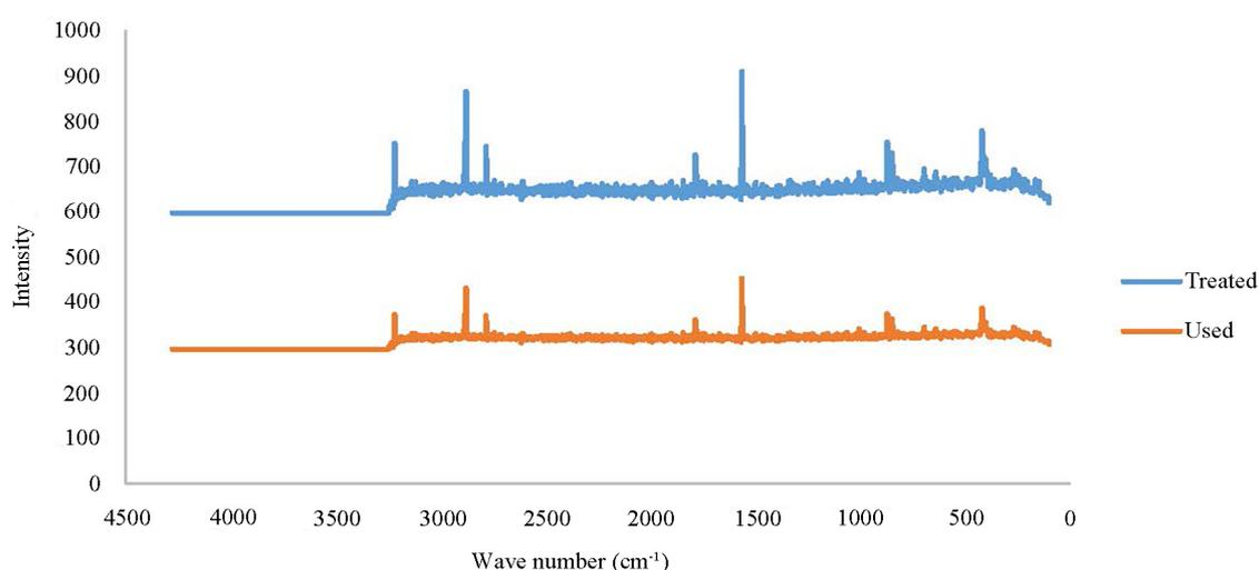
**Figure 4.** Combined Raman spectra of used and treated feldspar adsorbent
