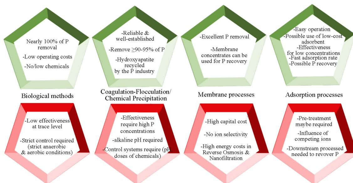
**Figure 1.** Synopsis of different approaches for Phosphate removal and recycling from wastewater, modified<sup>11</sup>
