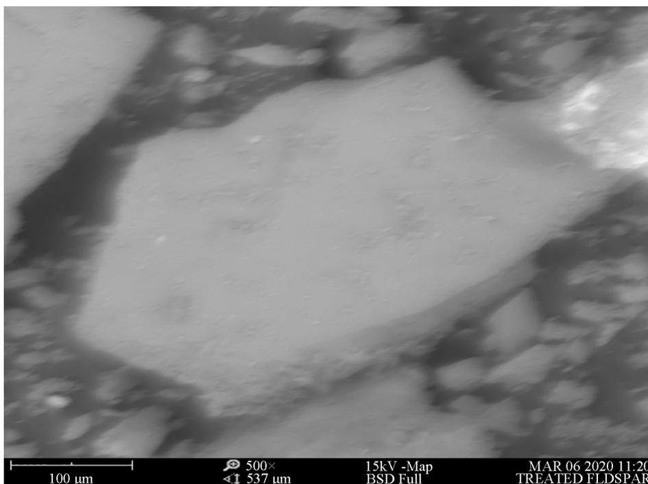
**Figure 8.** SEM of treated feldspar adsorbent at a magnification of (500X)
