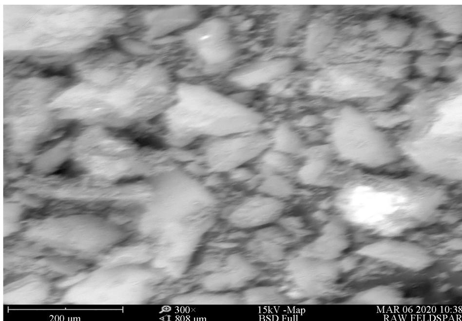
Figure 5. SEM of raw feldspar adsorbent at a magnification of (330X)
